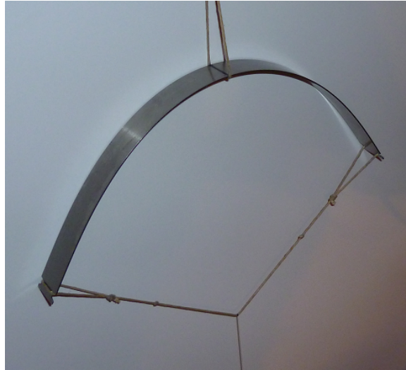
Figure 5.1: Steel bow. Cross section: 16.85 \times 0.75\text{mm} . Length: 269mm. Brace height: 49.8mm
